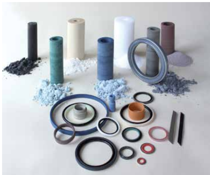
Fig. 1.3 PTFE powder, semi-finished shape and final machined product
